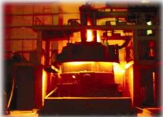
Ladle Refining Furnace
